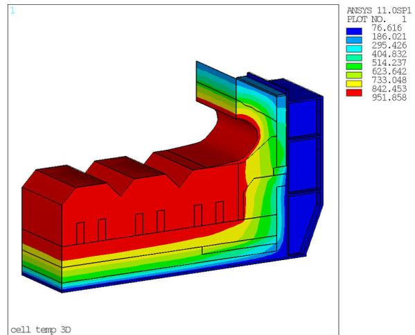
Figure 7. New thermal insulation lining structure, pot end temperature
