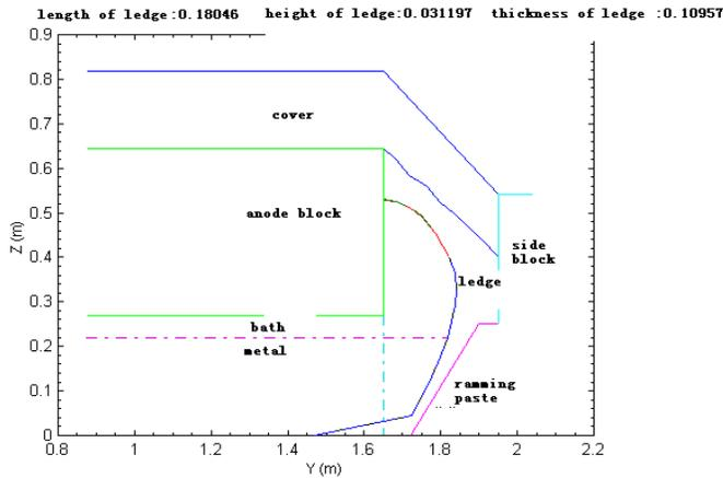
Figure 8. Conventional lining structure, profile of pot side ledge
