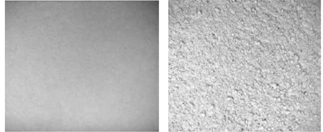
**Figure 1. Covering materials sample with above 93% Al<sub>2</sub>O<sub>3</sub> left, covering materials sample with below 13% Al<sub>2</sub>O<sub>3</sub> and 0.5-8mm bath crushing size right**
