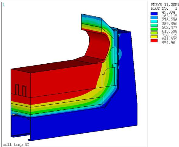
Figure 4. Conventional lining structure, pot side temperature
