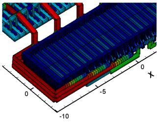
Figure 15a. Geometry of the 500 kA with transversal ridges case model (BARSIN and BUSNET files)
