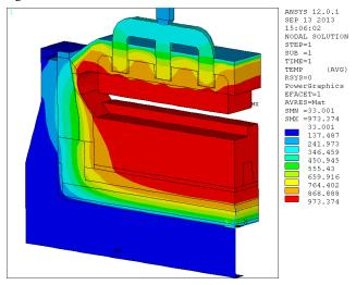
Figure 8. Full cell side slice thermo-electric model thermal solution with a transversal ridge
