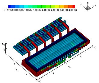
Figure 11. Geometry of the 500 kA base case model showing the current intensity solution in each conductor in A
