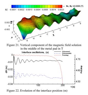
In a short time after the beginning of the simulation, the bathmetal deforms and touches the anode, stopping the simulation so that configuration is predicted to be unstable.
