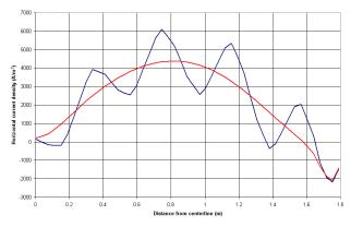
Figure 7. Comparison of the current density in the metal pad, with and without ridges, in A/m<sup>2</sup>
