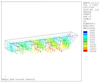
Figure 6. Current density in the metal pad in  $A/m^2$
