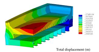
Figure 3. Cathode panel displacement results from thermomechanical potshell and lining modeling
