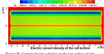
Figure 20. Current density solution on the top surface of the cathode in  $A/m^2$
