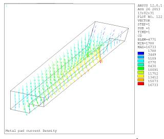
Figure 10. Current density in the metal pad in A/m<sup>2</sup>
