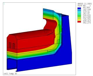
Figure 1. Example of irregular top surface cathode design
