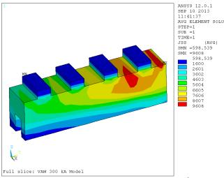
Figure 5. Current density in the cathode block in A/m<sup>2</sup>
