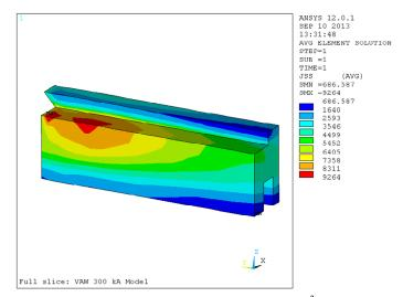
Figure 9. Current density in the cathode block in  $A/m^2$
