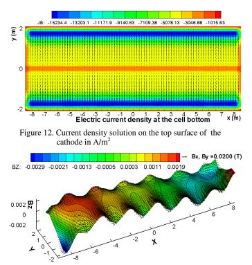
Figure 13. Vertical component of the magnetic field solution in the middle of the metal pad in T
