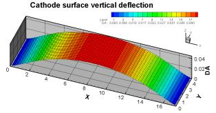
Figure 2. Metal pad bottom profile input for an impact of cell deformation cell stability study
