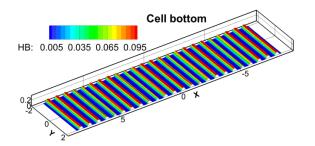
Figure 15b. Geometry of the 500 kA with transversal ridges case model (BOTTOM file)
